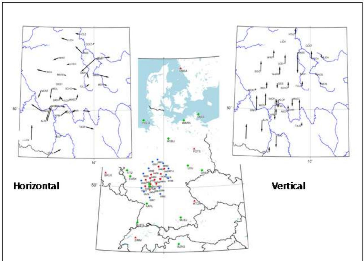
Figure 3. Horizontal and vertical station velocity vectors of the German Federal Network SAPOS-Hessen from re-processing
